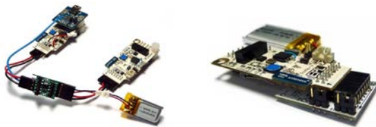
(a) Current sensor. (b) Battery fuel gauge.
