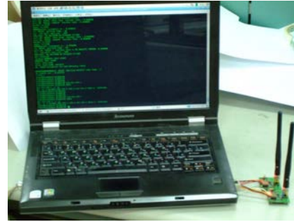
Fig. 6. A substitute gateway node implemented with a Linux laptop equipped with two transceivers for experimental setup.
