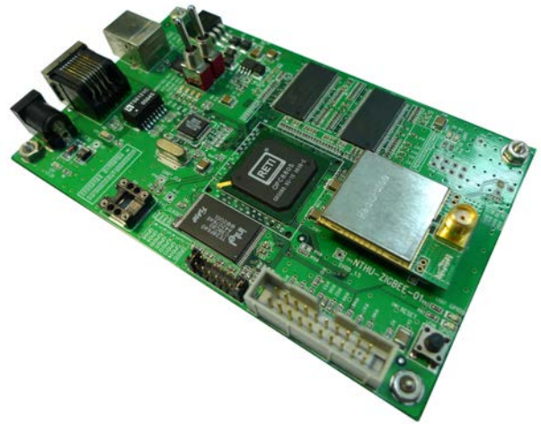
Fig. 1. The fully assembled EZ-Gate board.
