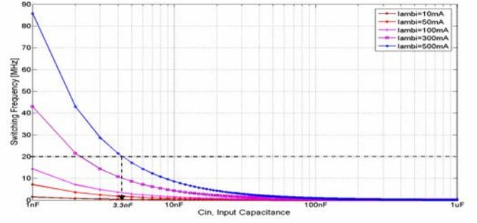
Fig. 8. Variation of switching frequency for different  $C_{in}$
