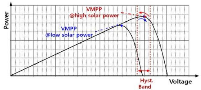
Fig. 2. P-V Characteristics and Hysteresis Window of the MPP
