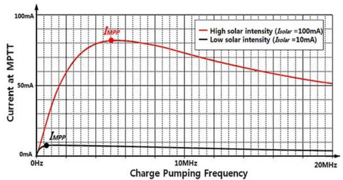
Fig. 10. Sweeping Frequency and Current for MPTT.
