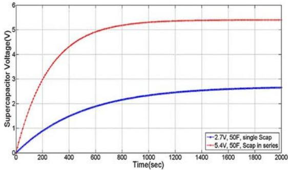
Fig. 9. Comparison of voltage over time for charging supercapacitors.
