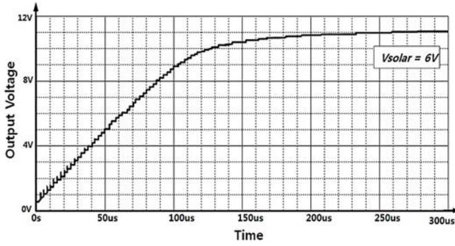
Fig. 7. Boost-up voltage of the Charge pump.
