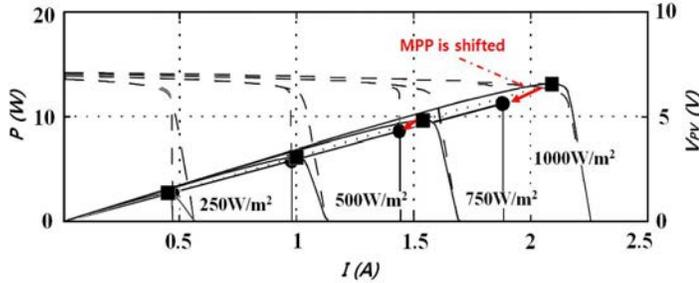
Fig. 1.  $MPP_{scap}$  vs.  $MPP_{solar}$ , when  $P_{scap} = \eta \cdot P_{ambi}$ . [7]
