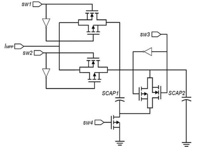
Fig. 6. Smart Switch Array for SCAP connection.
