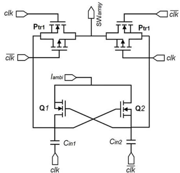
Fig. 4. Charge pump cell.
