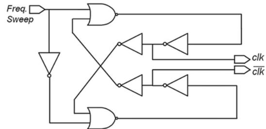
Fig. 5. Non-overlapping Clock controller.
