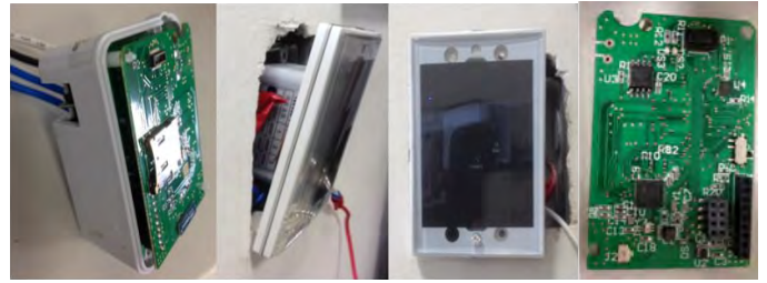
Fig. 5: Light Controller with touch panel.
