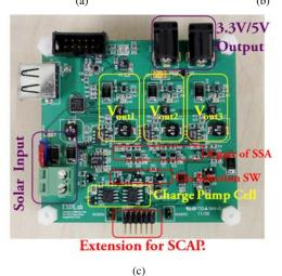
Fig. 4. (a) EscaCap prototype (b) supercapacitor modules (c) top view
