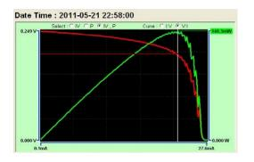
Fig. 5. Measured Solar panel I-V curve.
