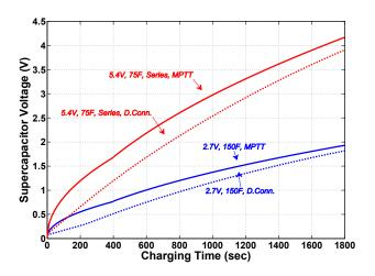
Fig. 8. Measured voltage over time for charging supercapacitors with solar power from Fig. 5. Solid lines: MPTT; dotted lines: no MPTT; red (upper two curves): two in series; blue (lower two): single supercapacitor.
