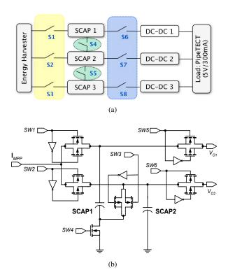
Fig. 3. Dynamic reconfigurable switch array (DRSA): (a) block diagram for three supercapacitors, (b) schematic for two supercapacitors
