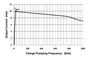
Fig. 7. Sweeping Frequency and Current for MPTT.
