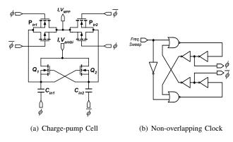
Fig. 2. Charge Pump Configuration
