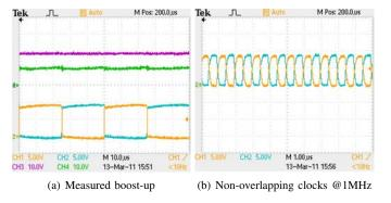
Fig. 6. Measurement of charge-pump operation.
