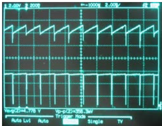
Figure 3: PFM Regulator Waveform: V_{solar} (top), S_2 (bottom)
