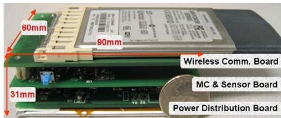
Figure 7: A photo of the DuraNode wireless sensor system.
