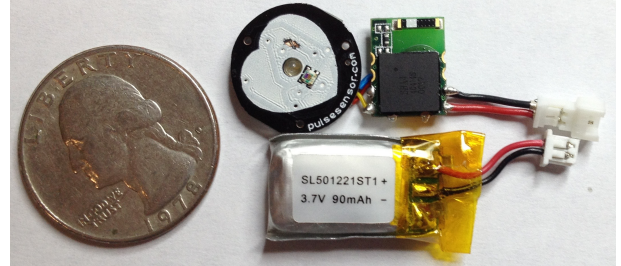
Fig. 1: Proposed hardware system. Top left: optical sensor board, top right: BLE and MPU-9250 board, bottom: battery.
