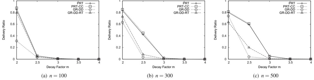
Fig. 9. Path Loss Coefficient  $m$  vs. Delivery Ratio
