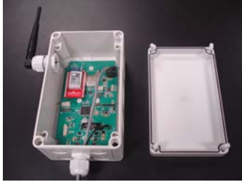
Fig. 8. The Aggregation Unit with WiFi attached
