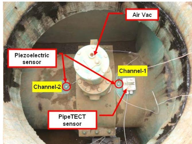
Figure 5. Installation of piezoelectric accelerometers
