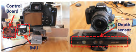
Figure 1. The system picture: The system is composed of DSLR camera (Canon EOS450d with 18-35mm lens), IMU (Analog devices, ADIS16350), Depth sensor (Microsoft Kinect), and Control board (Beagleboard-xm)
